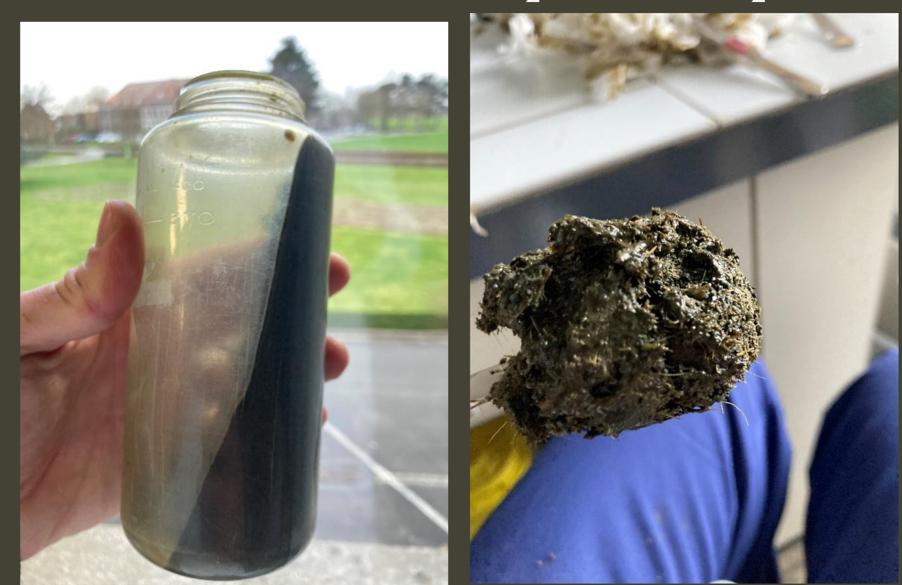
Fig. 6: Left: liquid fraction. Right: solid fraction after separation of the slurry
